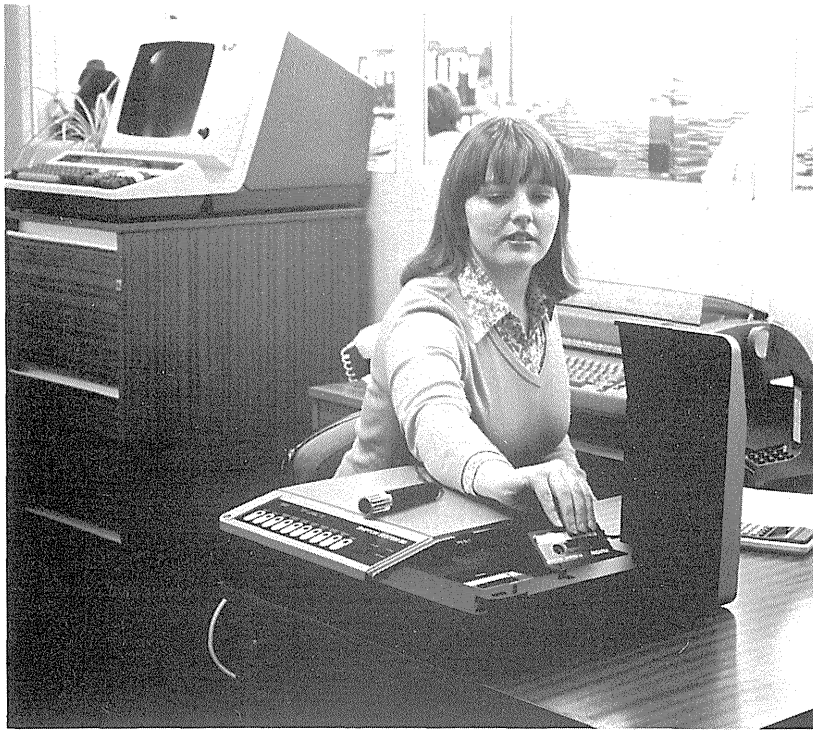
45 A telephone answering system which can be used for the remote control of office equipment and for automatic contact between offices over long distances, made by Shipton Communications Ltd.
