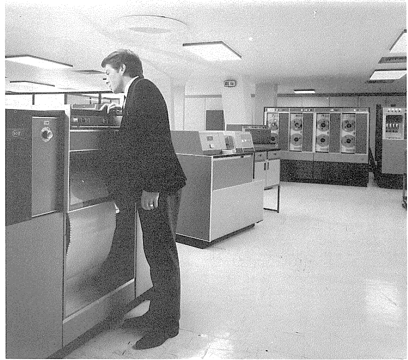
8 Part of an ICT 1900 series computer built in the mid-1960s using integrated circuits.
