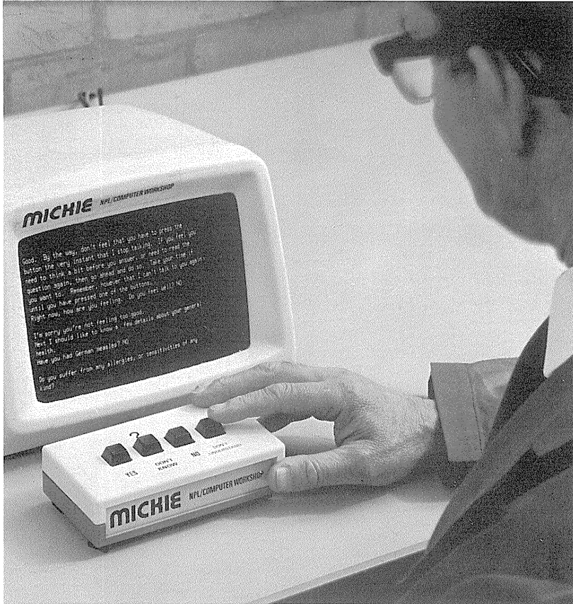
50 'Mickie' developed by the National Physical Laboratory and produced by Computer Workshop Ltd can help people to diagnose their own complaints.
