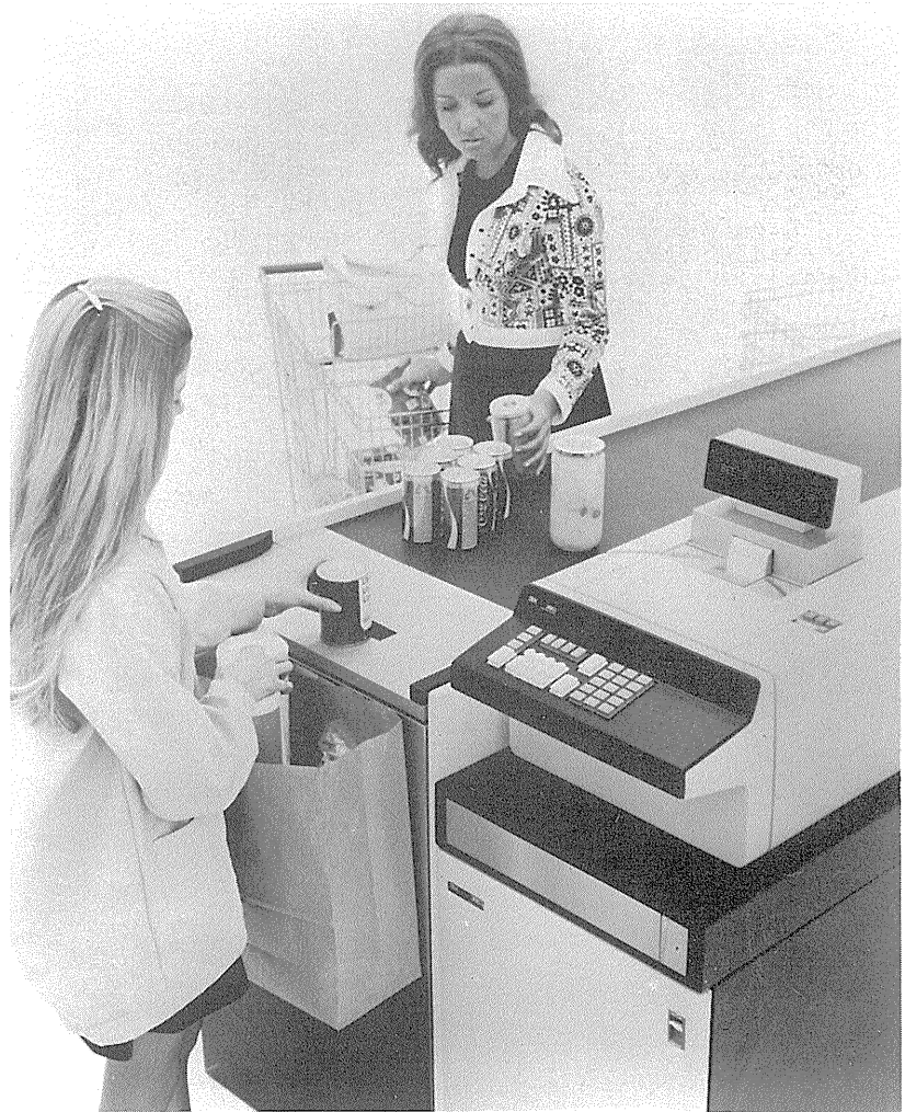
44 Products are priced and totalled automatically at this supermarket check-out point developed by IBM.
