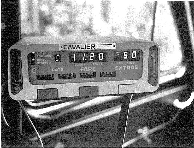
52 A microelectronic taximeter—introduced by three taxi service operators who were dissatisfied with the traditional meter.
